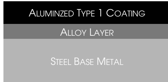
FIGURE 1- COATING CROSS SECTION*
